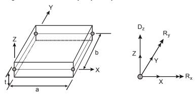
Figure 2-4 The Plate Finite Element
