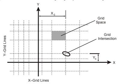
Figure 2-2 The Reference Grid System
