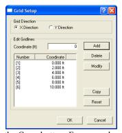
they are mirrored in the other direction, choose the COPY button. For example, if you just finished defining the grid lines in the X-Direction then the COPY button will copy all X-grid lines to Y-Direction.
