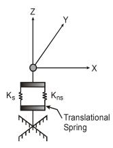
Figure 2-5 The Soil Element
