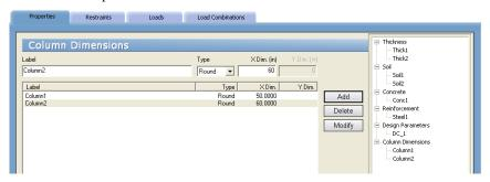
Enter a label or Column ID in the LABEL text box and select the TYPE of COLUMN (Round or Rectangle) from the drop-down list.
